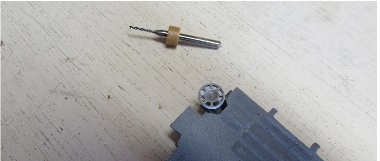
13. The mounting bracket: Clean up the flash. If you want the brake wheel in the lowered position, drill a #56 in the top of the bracket for the brake wheel. If you want the brake
