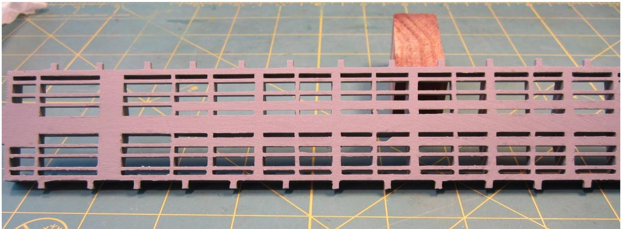
3. Invert the frame and add any brake detail you might desire. Since the car rides fairly low this isn't a requirement. The photo shows some basic detail that has been added. In these photos the brake wheel (notch in the end of the frame) is on the left.
